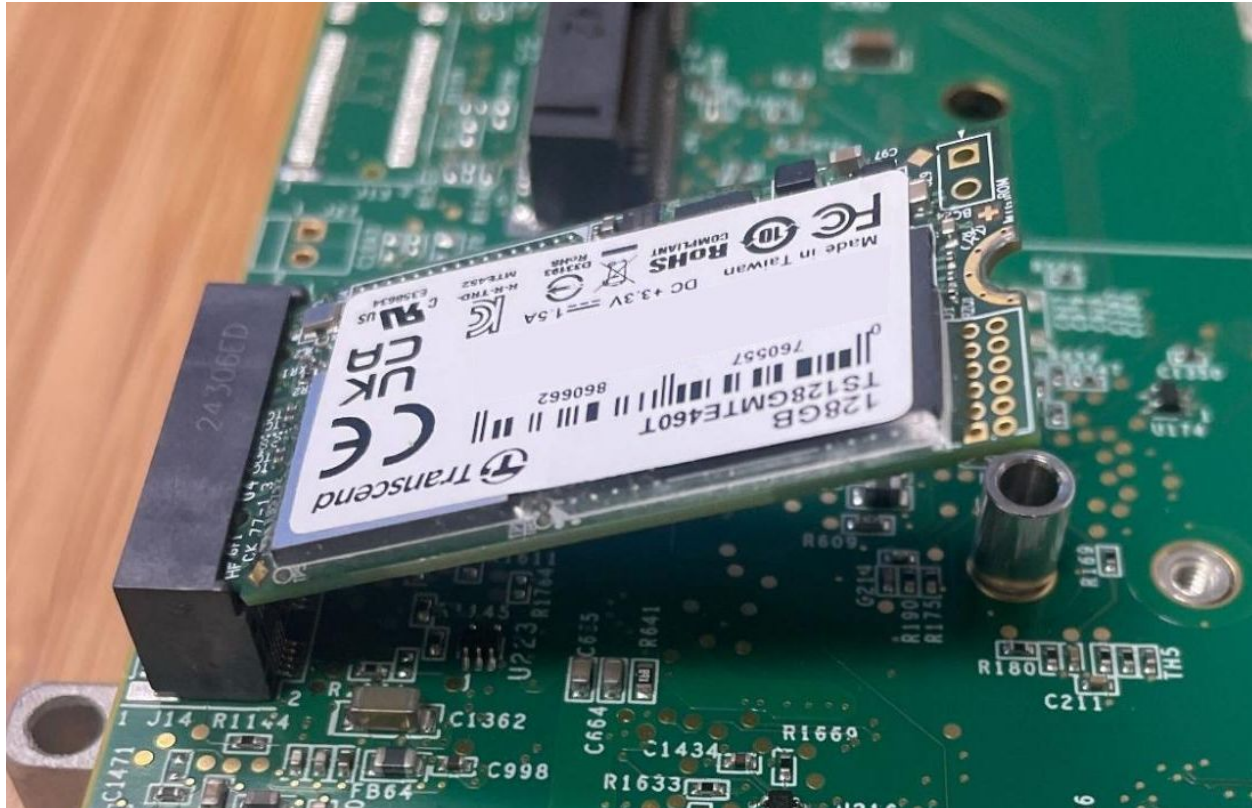
Fig. 31: Inserting the SSD into the M.2 socket at an angle
