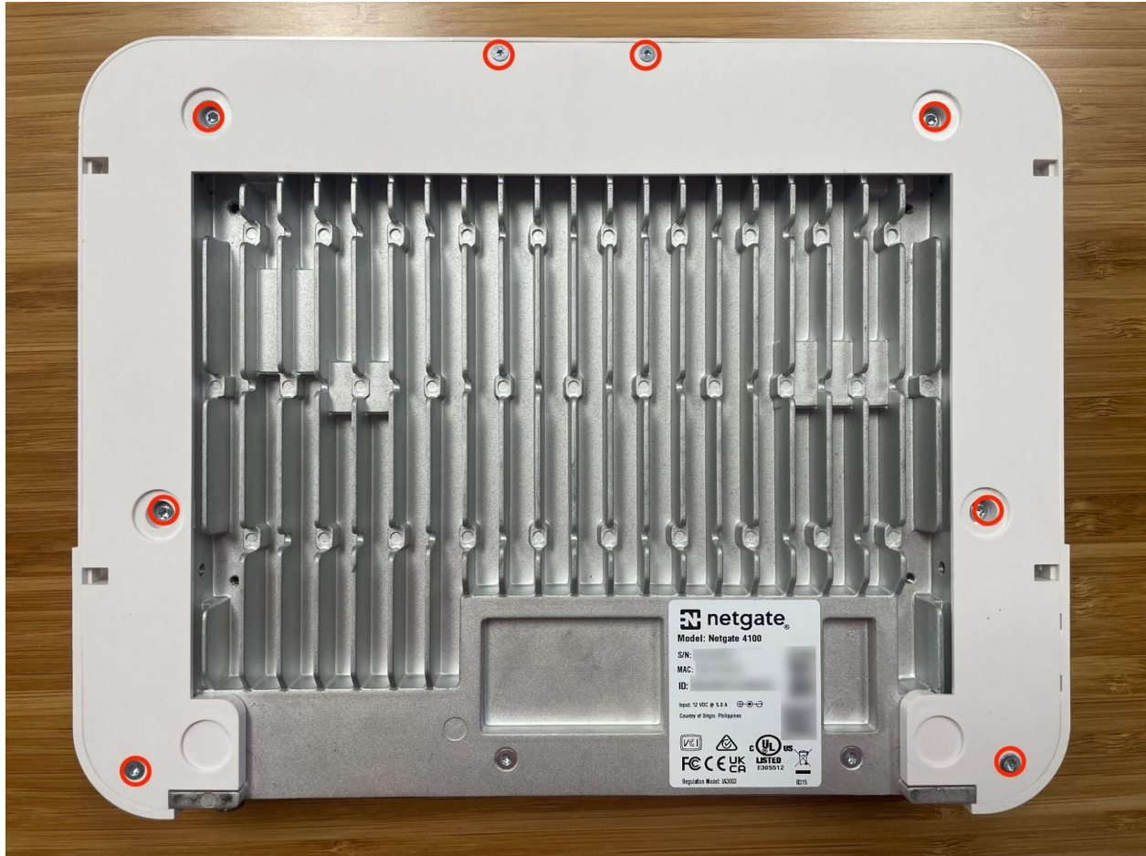
Fig. 35: Netgate 4100 case screw locations
