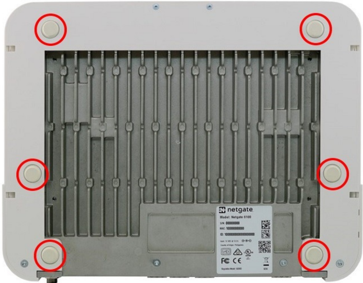
Fig. 6: Remove the Rubber Feet
