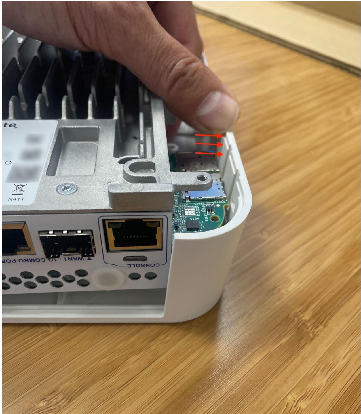
Fig. 34: Replacing the lid while clearing the SIM card slots
