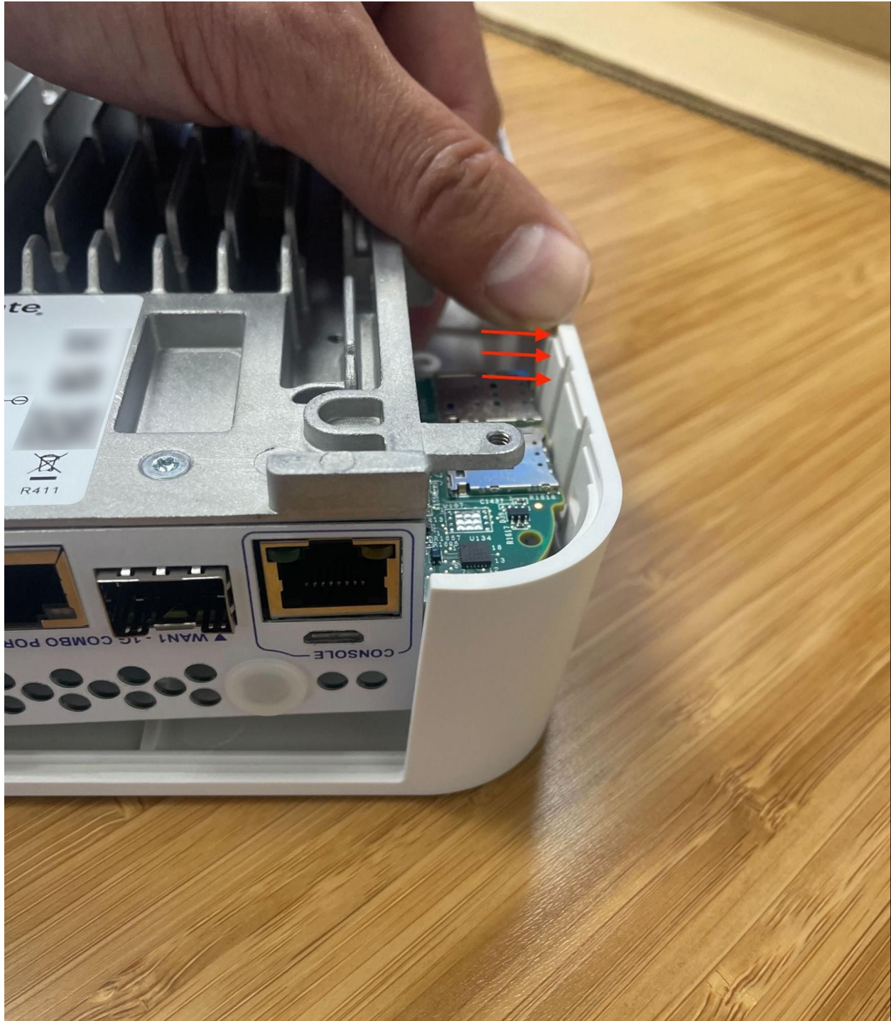
Fig. 28: Removing the lid while clearing the SIM card slots
