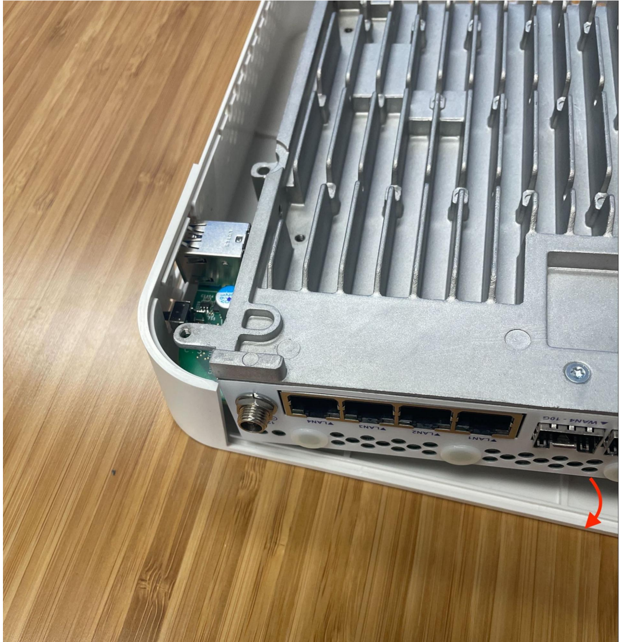
Fig. 33: Aligning the left edge of the lid with the USB ports and I/O panel
