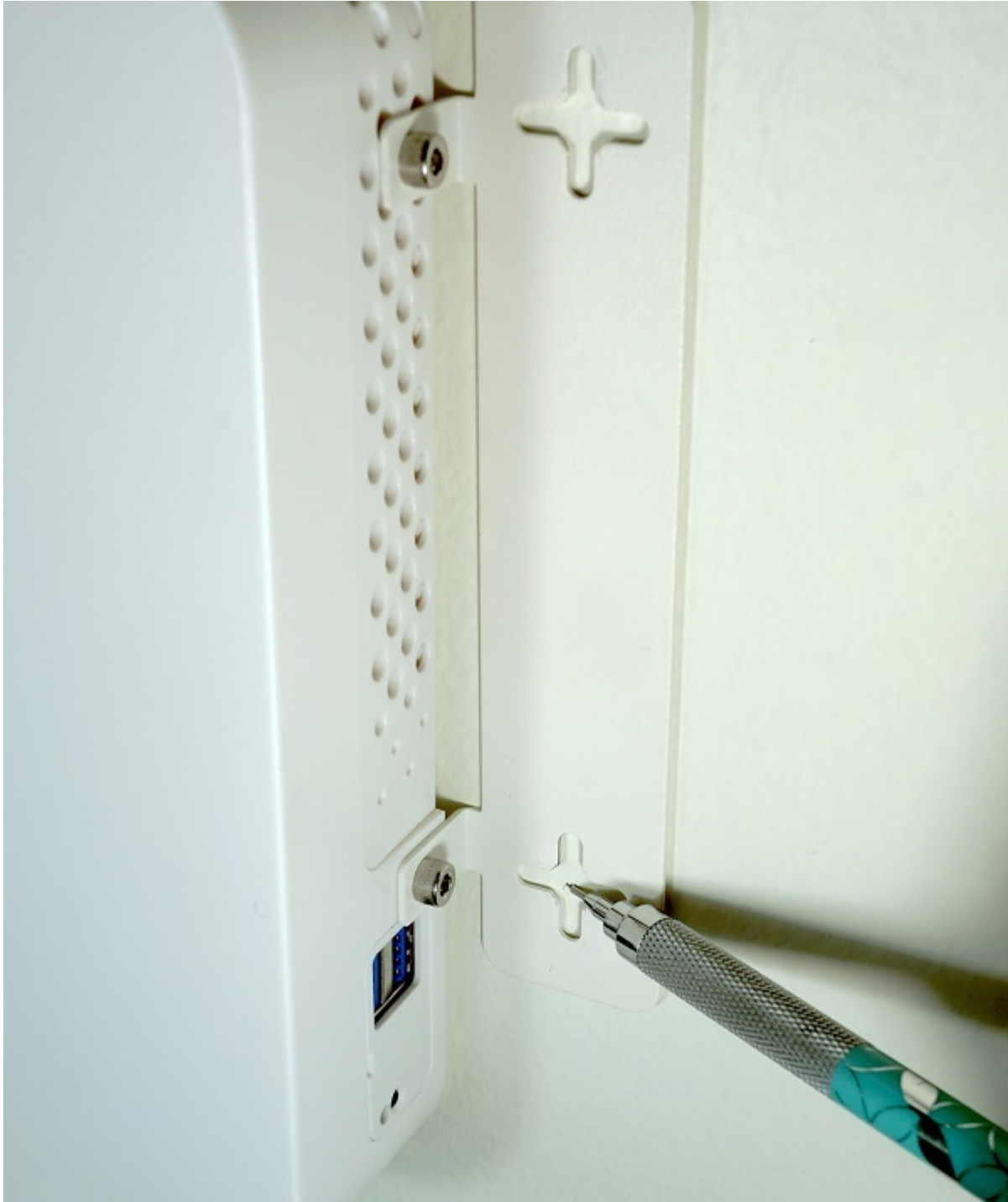
Fig. 20: Using the Netgate 6100 Wall Mount Bracket to Mark the Screw Locations
